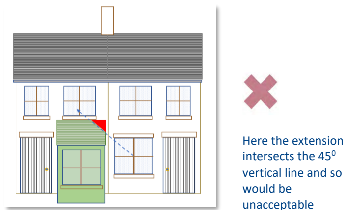
Figure 11: The 45° Rule diagram – front view
